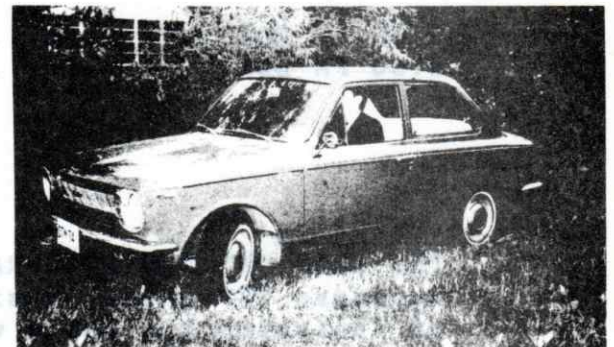
NEWEST IMPORT from Japan's No. 1 auto maker, Toyota, is the Corolla 1100, featuring a watercooled, 4-cyl. engine rated at 60 hp.
